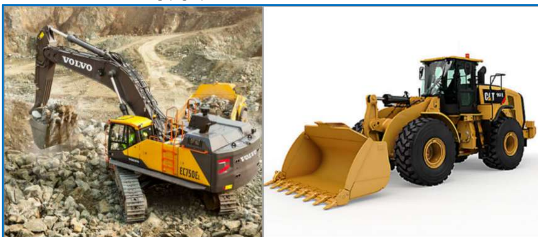
Figure 16-8: Loading Equipment: Backhoe Excavator for primary mining (left); FEL for re-handling (right)
