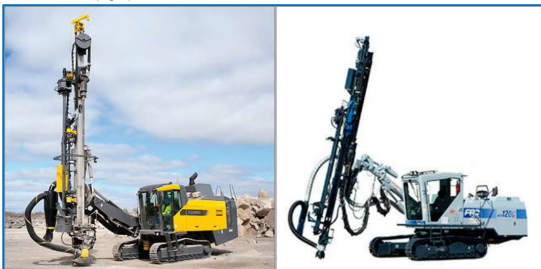
Figure 16-7: Drilling Equipment: DTH for the waste (left); Top-hammer for the ore (right)
