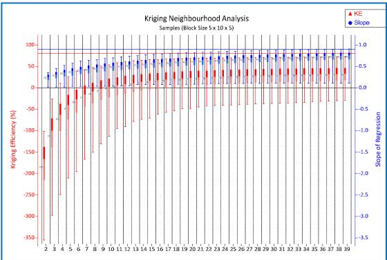
Figure 14-15: Change in kriging efficiencies and slope of regression with sample size
