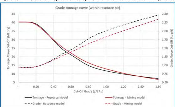
Figure 15-2: Grade tonnage curve – comparison of resource model and mining model
