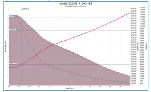
Figure 14-26: Grade tonnage curve for Posse 2020 Mineral Resource
