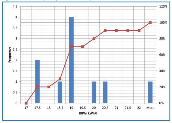
Figure 13 21 presents a plot of the BBWi determinations at the different product sizes. A strong relationship is shown. When attempting to estimate the 50th percentile from the histograms, the histograms require interpolation. It can be interpreted the 50th percentile values for the
