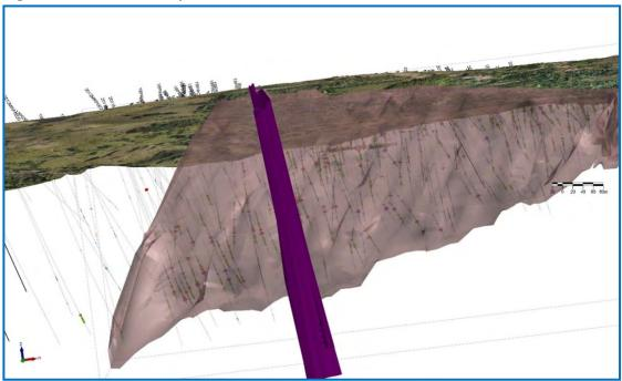
Within the Z3 mineralized domain it was possible to trace near continuous nested zones of higher-grade mineralization. These were defined by the same process as that adopted for the Z3 mineralized domain. For this model grade zones representing a 0.5g/tAu (Z2 domain) and a 1.0g/tAu (Z1 domain) were generated as shown in Figure 14-6.
