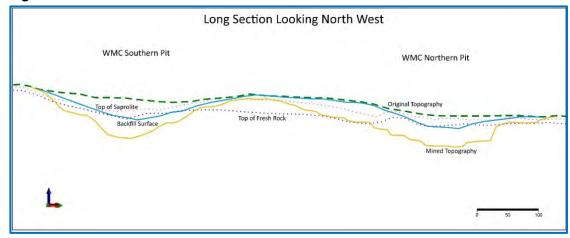
Figure 14-8: Surfaces used to control zonation in the block model
