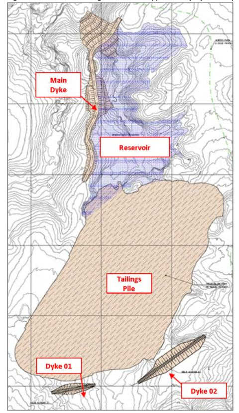
Figure 18-6: Filtered Tailings Pile Area for approximately 2 years of operation
