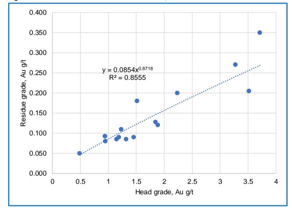
Figure 13-29: Residue Grade versus Head Grade, 36 hours
