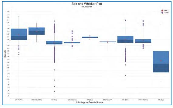
Table 12-13: Comparison of density readings by rock type<sup>(1)</sup>
