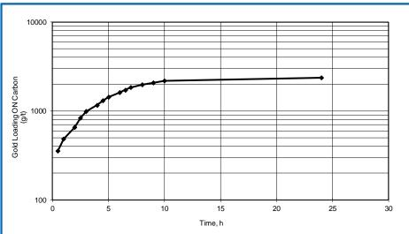
Figure 13-26: Detox Composite Carbon Kinetics 6 x 12 mesh
