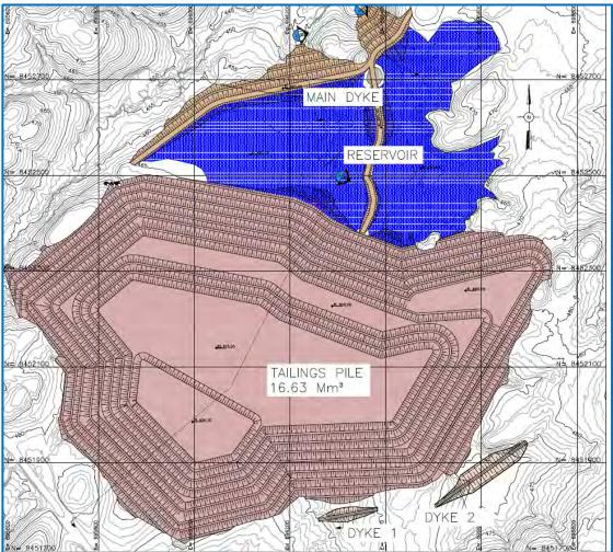
Figure 18-7: Filtered Tailings Pile Final Area
