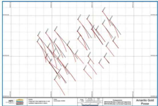
Figure 12-1: Holes from 2011 drilling with incorrect downhole survey
