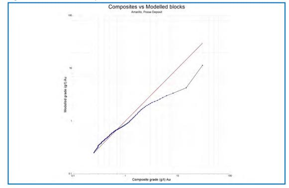
Figure 14-22: QQ Plot composites vs modelled blocks
