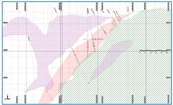
A late, un-mineralized basaltic dyke, which had been encountered in a number of drillholes, was modelled and incorporated as a separate wireframe, which transects the Posse mineralization. In earlier models this dyke was not well defined and there were concerns about its effect of the volume of mineralisation. Current modelling indicates that this dyke, Figure 14-5, is thin and has negligible effect on the mineralized volume.
