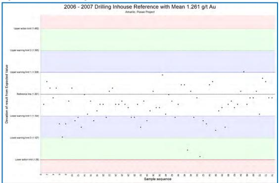
Figure 12-6: 2006 Drilling, Standard 1a, Shewhart Plot
