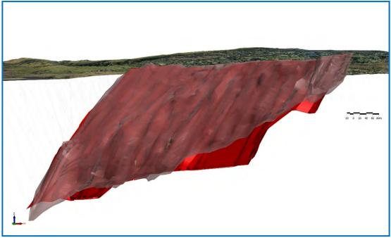
The mineralization is largely confined to the schistose zone which is situated between a Biotite Gneiss hanging wall and the Amphibolite footwall, Figure 14 4, drill results indicate that the hanging wall and footwall units are discontinuous and there appears to be potential for repeats of these structures.
