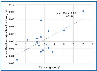
Figure 13-31: Residue Grade versus Head Grade, 36 hours
