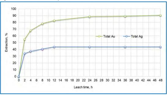
Figure 13-14 is directly comparable to Figure 13-13 to understand the potential benefit of pH influence. Figure 13-14 presents the kinetics for the leach at pH 12.5 without pre-oxygenation. The plot reveals the most rapid leach kinetics of all of the tests presented by the four graphs. However, the long leach tail as observed in the pre-oxygenation tests remains with a slow but consistent leach rate presented between 12 to 48 hours.
