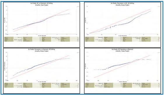
The second set of images, Figure 12-14, shows comparisons between the same type of sampling and the company that carried out the drilling. All comparisons show a good relationship between datasets:
