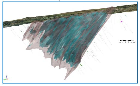
Based on the current geological information in the drillhole database, which contains limited information, there is no obvious geological basis for these domains. However, work by MINCON for Amarillo in 2003 using geological interpretations developed by MBL noted higher grades associated with more intense shearing and more importantly increased silicification and
