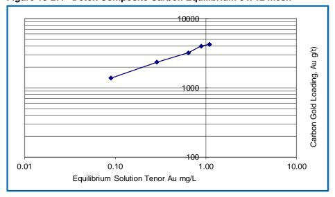
Kinetic and equilibrium parameters as determined from the test work are presented as:
