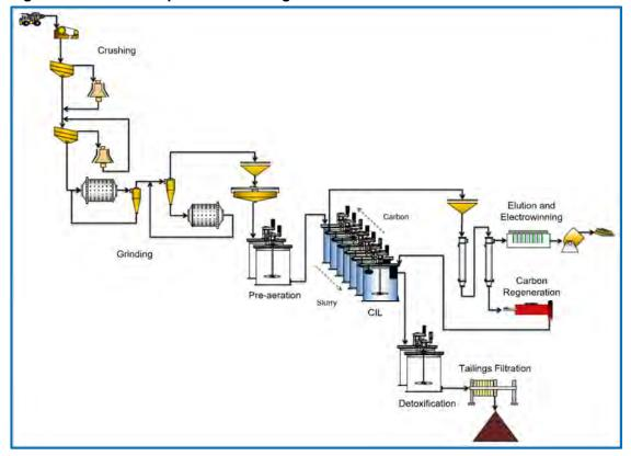
Figure 17-1: Overall process flow diagram
