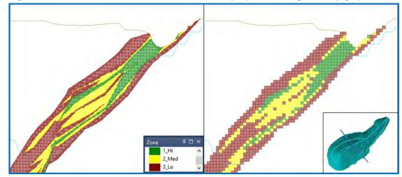
Figure 15-1: Vertical section of resource model (left) and mining model (right)
